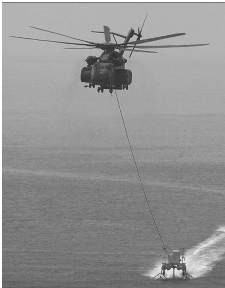
ARABIAN GULF — An MH-53E Sea Dragon helicopter tows a MK-105 Magnetic Influence Minesweeping System or 'sled' during operations with USS Saipan in the Arabian Gulf in September 2006. Saipan was on deployment to the region conducting maritime security operations, ensuring security and safety in international waters so that all commercial shipping can operate freely while in the region. Photo by MC2 Steven J. Weber
