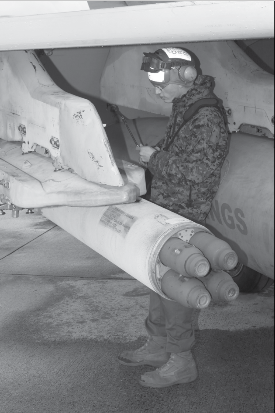
KADENA AIR BASE OKINAWA, Japan — Lance Cpl. Casey Hayes, Marine All-Weather Fighter Attack Squadron 225 aviation ordnance technician, ensures a launch adapter unit is safely secured to a VMFA(AW)-225 F/A-18 Hornet during a unit-level training exercise here Dec. 17. Aviation ordnance technicians ensure all ordnance is safely secured several times before a jet can take off.
