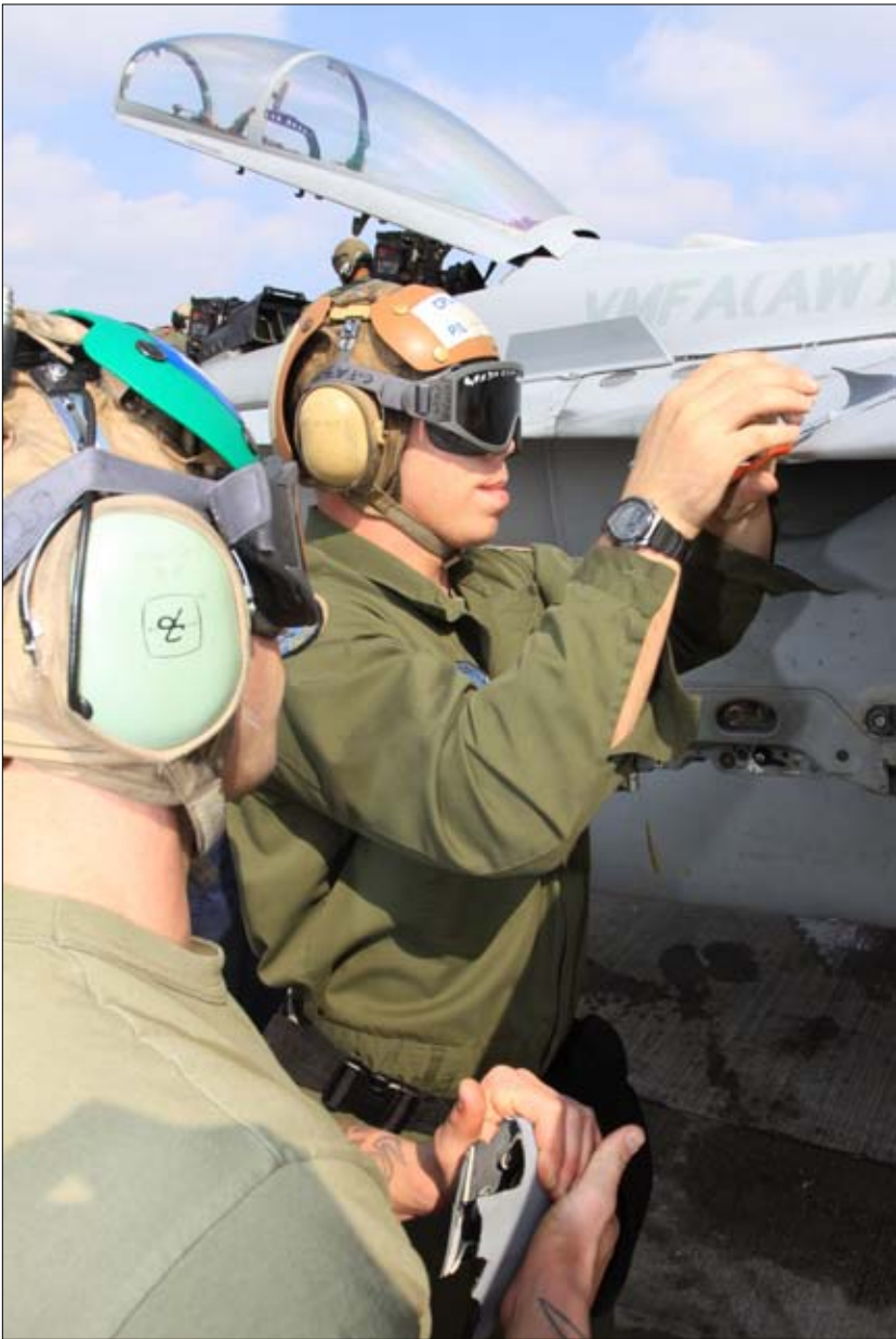
KADENA AIR BASE OKINAWA, Japan — Cpl. Joseph Williams, Marine All-Weather Fighter Attack Squadron 225 power line technician, removes a clamp shell from an aircraft to prevent TFOA (things falling off aircraft) during hot pit, hot seat training here Dec. 22.
