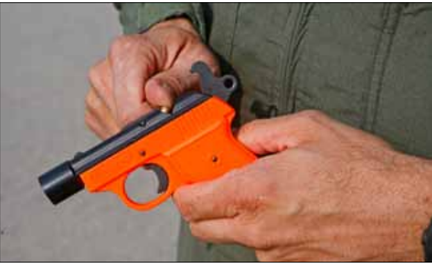
CPL. JOSEPH MARIANELLI Once armed with explosive propellant, a variety of noise makers can be placed on the muzzle of the pistol. When fired, the propellant will launch the noise maker into the sky where it will explode, making some awfully loud noise and hopefully scaring birds away.
