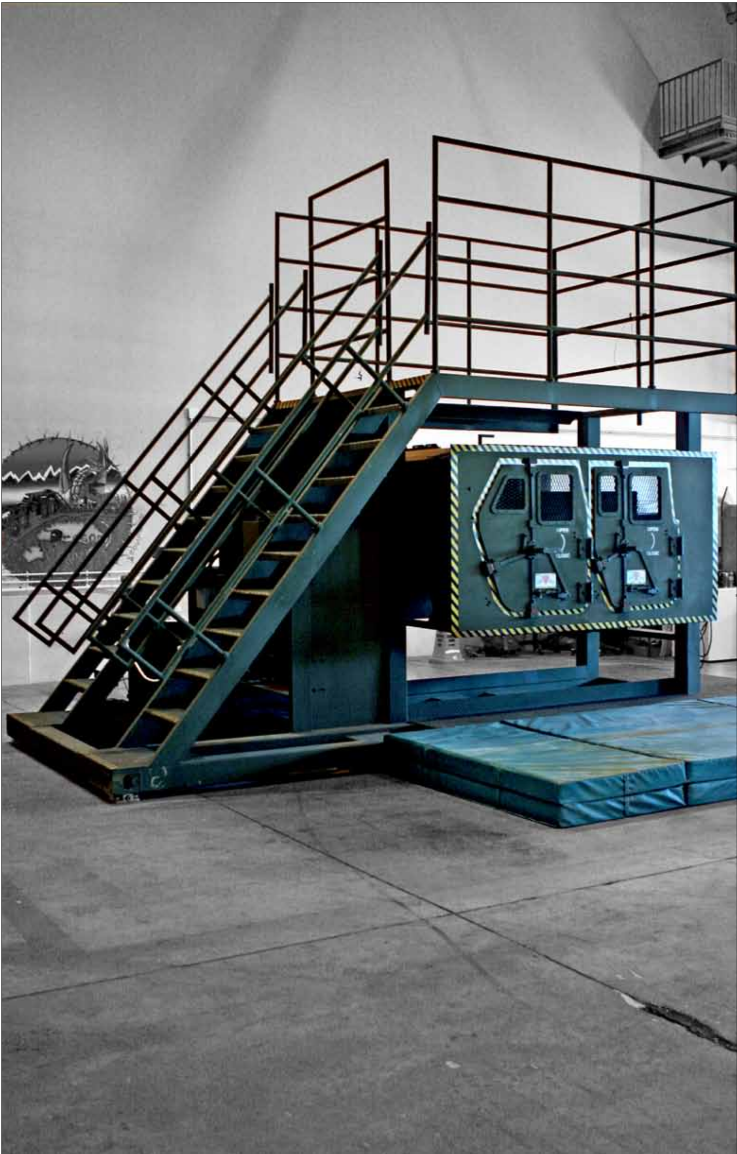
LANCE CPL. KENNETH K. TROTTER JR. The simulator used for Humvee Egress Awareness Training is part of the practical application portion of the HEAT course here Feb. 16. The machine was modeled after the cabin of a humvee and simulates the rolling motion of a humvee hit by an improvised explosive device. The course required the participating Marines to egress after the machine spins several times in rapid succession in under four minutes. The Marines were tasked with egressing either from the side hatches or the gunner's hatch.
