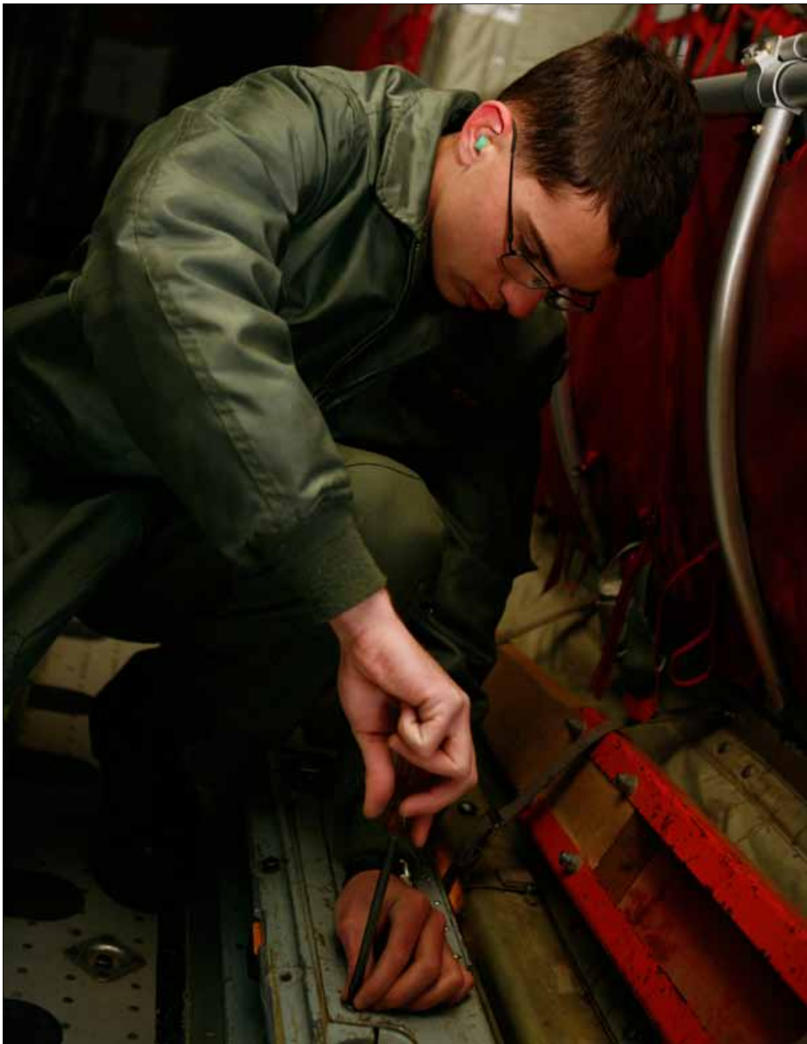
(ABOVE) Lance Cpl. Eric M. Wanczak, a Marine Aerial Refueler Transport Squadron 152 loadmaster, opens a panel so he can tighten one of the cargo locks necessary for keeping cargo pallets in place in preparation for a humanitarian mission to Sendai, Japan, as part of Operation Tomodachi here March 25. (BELOW) SENDAI, Japan – Lance Cpl. Eric M. Wanczak, a Marine Aerial Refueler Transport Squadron 152 loadmaster, and other crew members push water palletized at Marine Corps Air Station Iwakuni, Japan, out of the C-130 during a humanitarian aid mission as part of Operation Tomodachi here March 25. During this mission the crew delivered three water pallets and two supply pallets.
