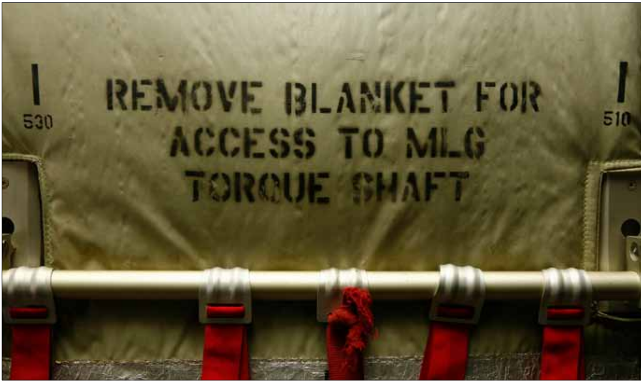
Hash marks indicate the number of inches from the nose of the aircraft in C-130s. Although C-130s are capable of transporting a payload of up to 45,000 pounds, the center of balance must fall between 512 inches and 536 inches or the aircraft will not be able to take off.
