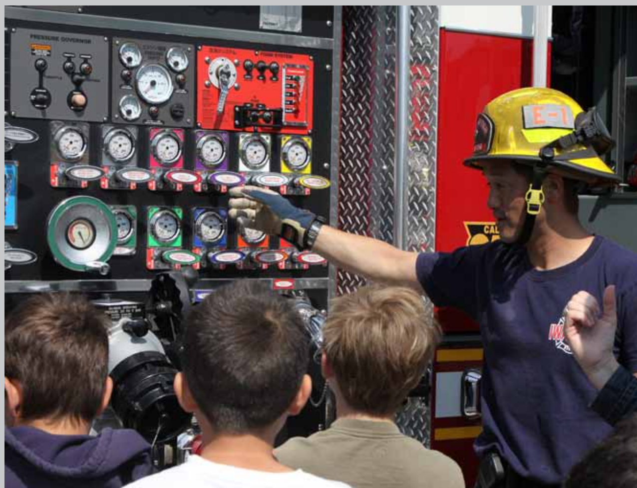
Ken Kobayashi, Marine Corps Air Station Iwakuni Fire Department firefighter, points out where all the hoses used to fight fires with connect to the water tank inside the truck at the Matthew C. Perry Elementary School playground here Monday. The hose attaches to the truck where the knob is pulled, filling the hose with water, allowing the fire fighters to shoot water at a fire. The MCAS Iwakuni Fire Department firefighters took time out of their day to visit the elementary school students and demonstrate their day-to-day job. The students listened in awe as they learned information about firefighting they did not know before.
