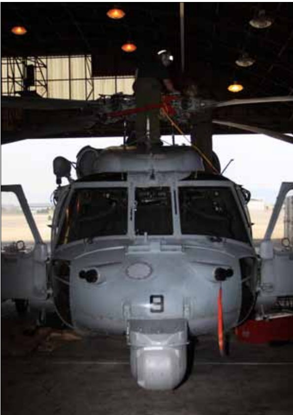
Two Helicopter Sea Combat Squadron 25 aviation electricians check the main rotor hub system of one of their MH-60S Knighthawk helicopters during a Phase D inspection at the HSC-25 hanger here June 6.
