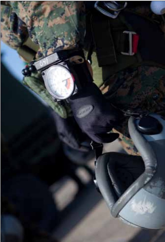
CPL JEFF DREW Marines with 2nd Reconnaissance Battalion, 2nd Marine Division, who participated in a free-fall sustainment jump, use an altimeter on their wrists to gauge the altitude at which to pull their parachutes. Jumping from a height of 10,000 feet means the Marines will pull their parachute at approximately 5,000 feet in order to safely return to the landing zone.
