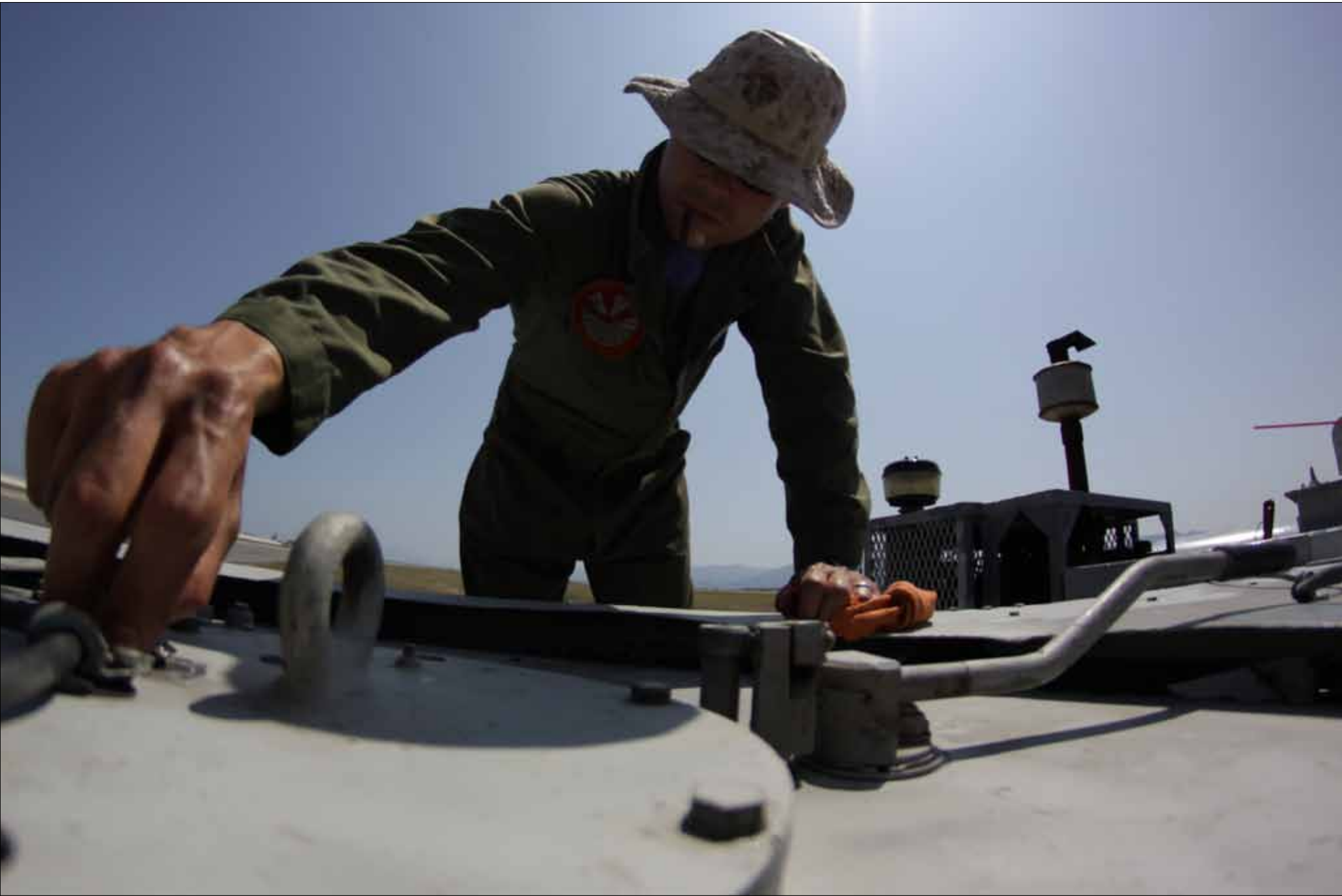
Lance Cpl. Benjamin Pryer Staff Sgt. Joseph R. Pacheco, A station runway supervisor, performs maintenance on an E-28 Emergency Runway Arresting Gear on the flightline, May 24, 2013. Recovery Marines perform daily maintenance checks, as well as any necessary work after the equipment is used.
