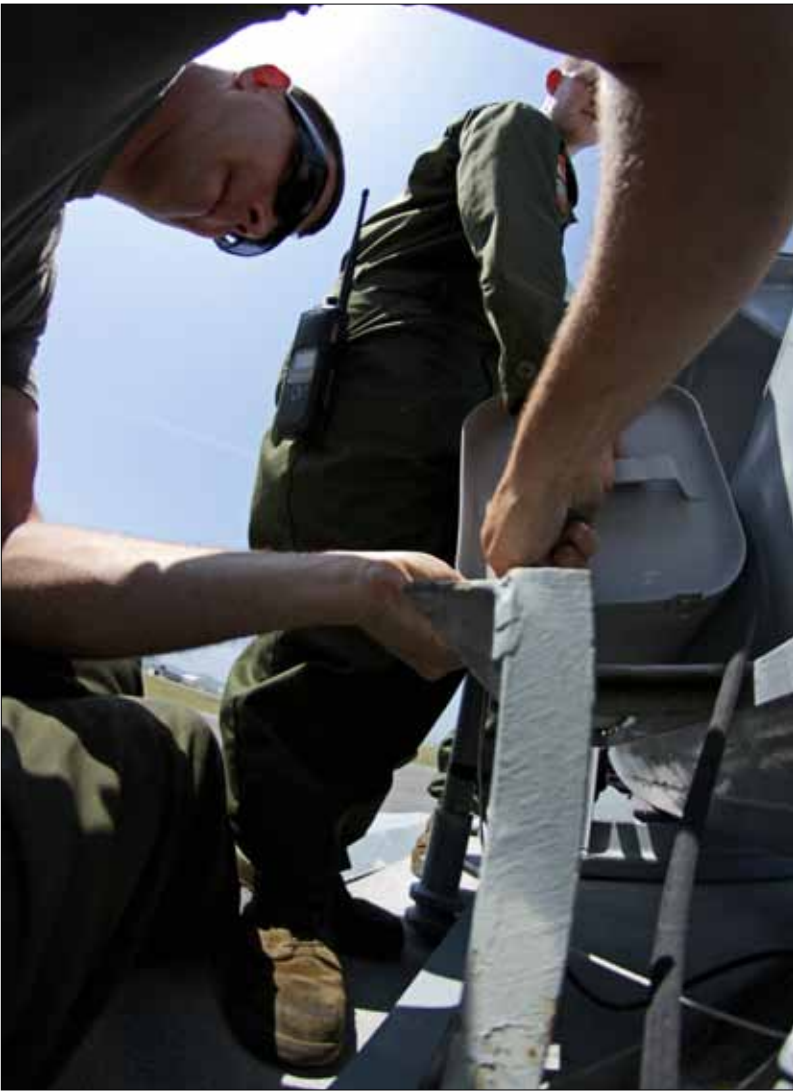
Lance Cpl. Benjamin Pryer Sgt. Blake Chaffin, A station aircraft recovery specialist, performs maintenance on an E-28 Emergency Runway Arresting Gear on the flightline, May 24, 2013. Recovery Marines must constantly ensure their gear is at peak performance in order for it to assist in an emergency landing.
