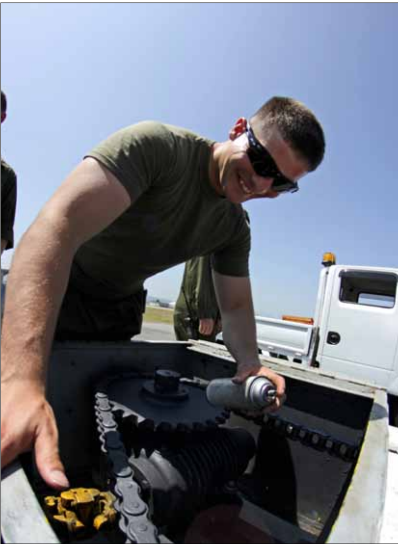
Lance Cpl. Benjamin Pryer Lance Cpl. Michael Truex, A station aircraft recovery specialist, performs maintenance on an E-28 Emergency Runway Arresting Gear on the flightline, May 24, 2013. Recovery Marines from Iwakuni also currently hold the military-wide record for arrestment landings conducted in less than an hour, performing 13 during Exercise Forager Fury 2012 .
