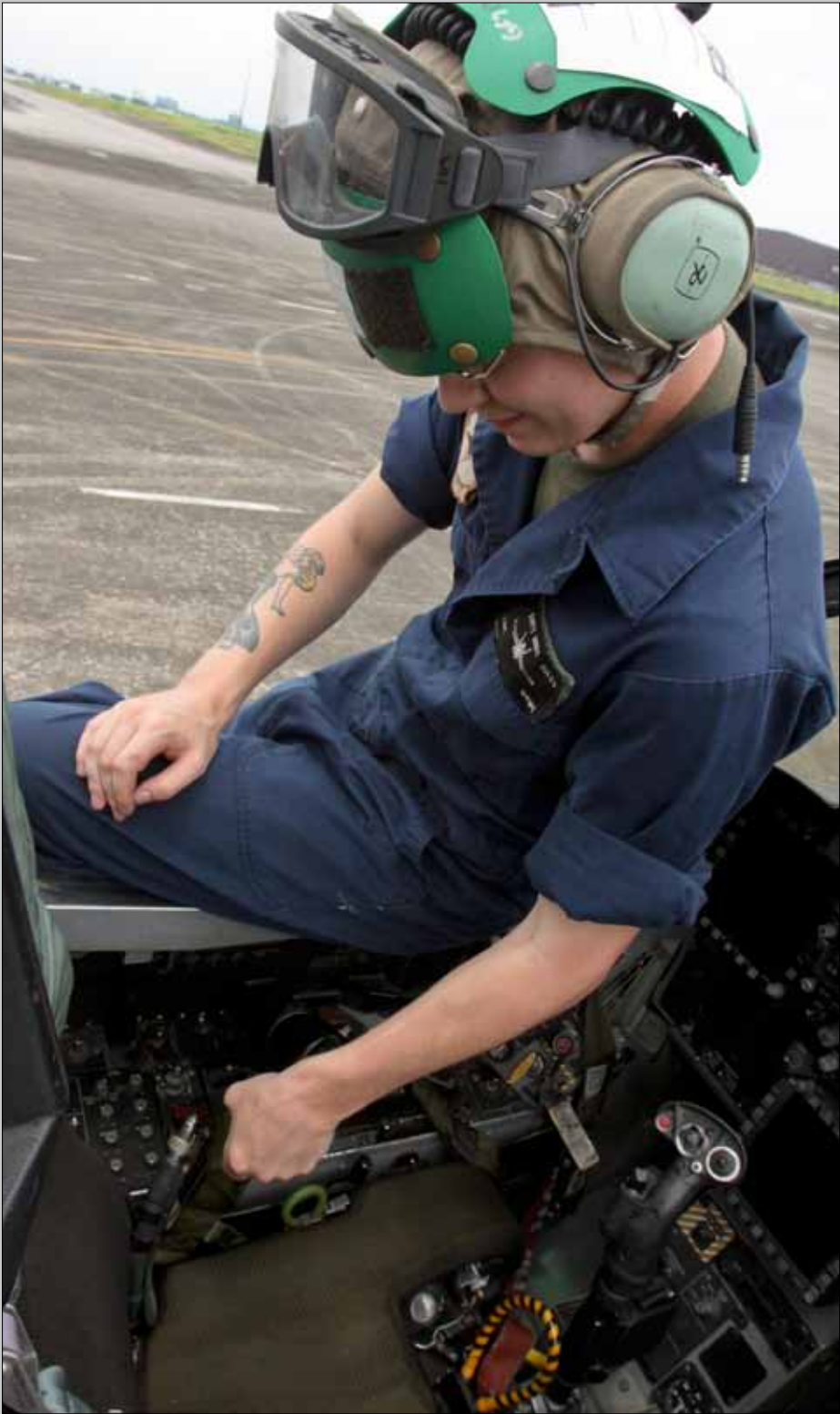
Lance Cpl. James C. Riley, A fixed-wing aircraft safety equipment mechanic with Marine All-Weather Fighter Attack Squadron 242, inspects the ejection seat of an F/A-18D hornet June 12 during Exercise Haribon Tempest 2013. Riley inspects, maintains and repairs the aircraft’s safety equipment and systems. The focus of HT13 is to improve tactical-level military proficiency and enhance U.S.-Philippine interoperability and combined abilities.
