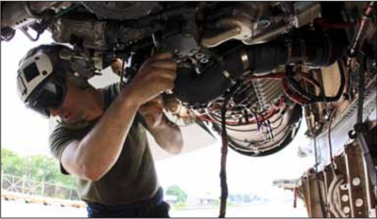
Sgt. Vincent T. Erzen, A fixed-wing aircraft mechanic with Marine All-Weather Fighter Attack Squadron 242, replaces a bleed air regulator in an F/A-18D Hornet at Clark Air Base, Republic of the Philippines June 14, during Exercise Haribon Tempest 2013.
