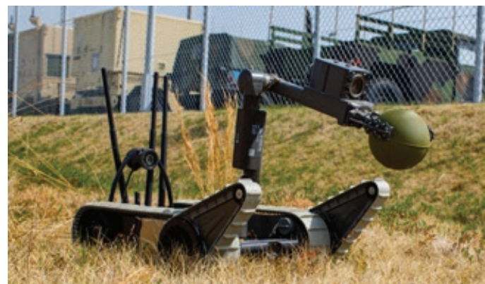
模擬子弾をつかむXM1216小型無人地上車両。 An XM1216 small unmanned ground vehicle grabs a simulated submunition.
