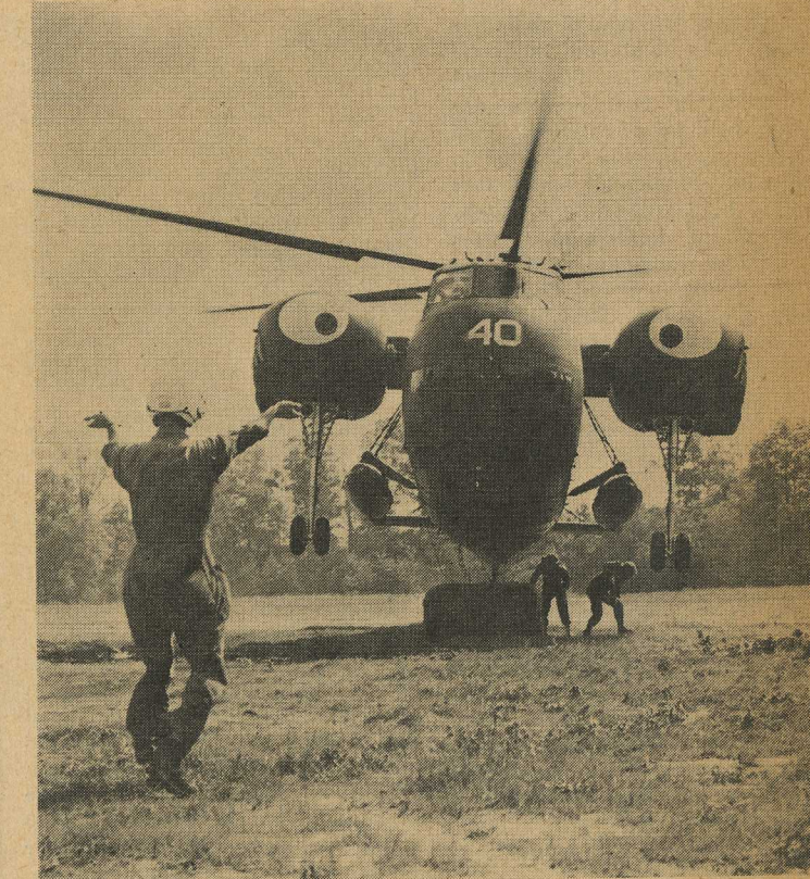
"MIGHTY MONSTER" -- A ground crewman directs a Marine Corps HR2S into position preparatory to the airlift of a 6,000-pound rolling container of fuel.
