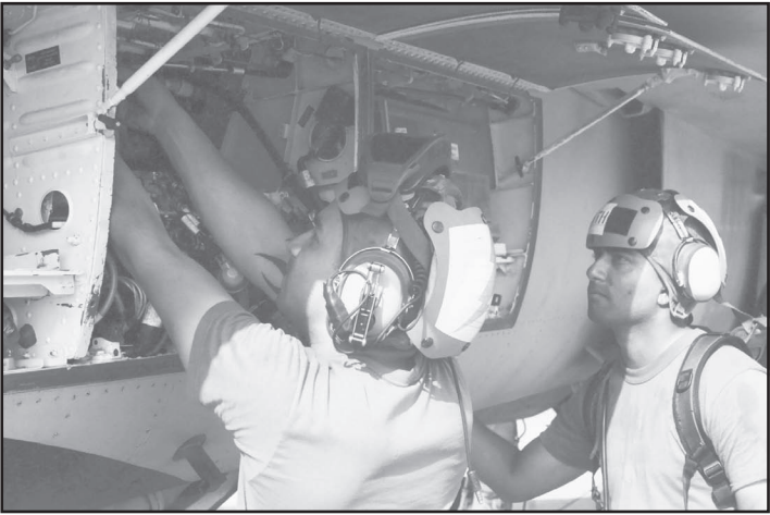
Cpl. Mauricio A. Driaza (left) and Lance Cpl. Jason A Ramnath, both VMFA-251 power line mechanics, replace a throttle boost actuator from a F/A-18D plane.
