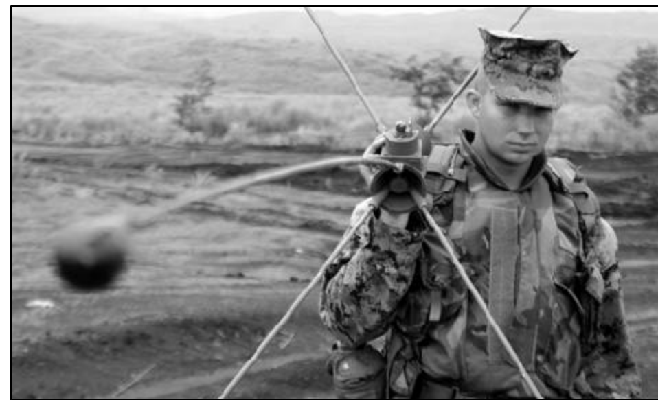
Lance Cpl. Eric Chase, MWSS-171 bulk fuels transporter, holds an OE-254 omnidirectional antenna which will be installed at the re-trans site here, June 19. The antenna helps provide the re-trans site with increased communications capabilities for the Marines during their two-week exercise.
