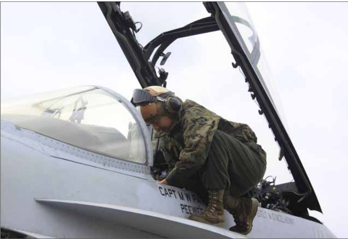
PFC. BENJAMIN PRYER A Marine with Marine All-Weather Attack Fighter Attack Squadron 242 checks the cockpit of an F/A-18 Hornet for maintenance for the surge day at the air field here Jan. 12. Even once all paperwork is finalized, the aircraft still needs to be checked before and after every sortie, ensuring all maintenance is up-to-date.
