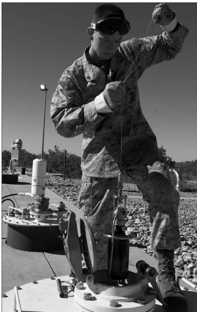
**Pfc. Travis Unwin pulls a fuel sample up from a tank atop fuel farm 2 here July 17. Samples are taken from each of the 14 tanks every day and tested by the base laboratory to ensure fuel quality. Photo by Lance Cpl. Joseph Marianelli**
